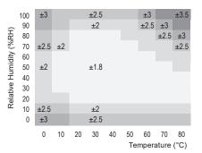
Figure 3. Typical accuracy of relative humidity measurements given in %RH for temperatures between 0 –  $80^{\circ}$ C.
